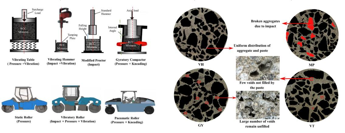
Compactors used for RCCP Design & Construction
